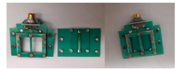
In this research, the signal was measured on the reference sample – a quantum well (Cd, Mn)Te with manganese content of 0.3%. The characterization was made based on measurements of various microwave radiation power and various environmental conditions, such as the temperature and pressure of helium surrounding the sample, affecting its dielectric constant. Obtained results are compared with the results of numerical simulations.
