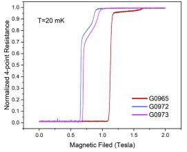
Superconducting to normal phase transition signatures for three Al layers: G0972 was deposited at 3.0 Å/s (10 nm thick) G0973 was deposited at 2.0 Å/s (10 nm thick) G0965 growth rate decreased from 2.0 Å/s to approximately 1.3 Å/s during the deposition
