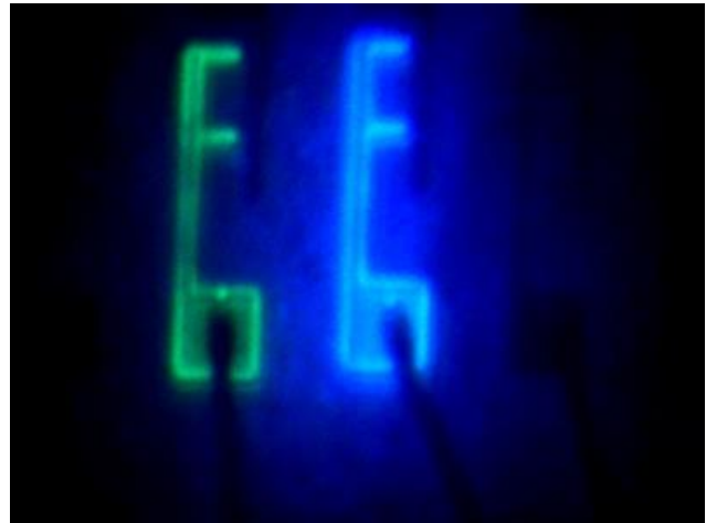
Fig. 1: Electroluminescence from two neighboring regions with different indium content on one of our devices. The change of wavelength can be clearly seen.
